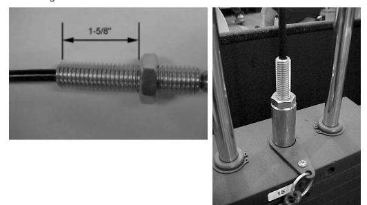
Figure 18. Screw the cable into the weight stack.
